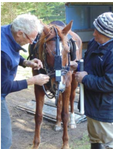
Figure 5a: Hanson attaching an audio-recorder to the exercise video-endoscope.
